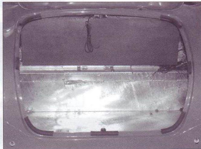
Left: Fig.17b. Fuel tank fitted. Shown here after the body has been fitted.
