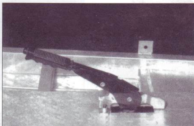
Fig.4b. Handbrake bracket bolted to transmission tunnel.
