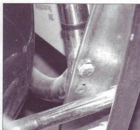
Fig.8e. Override bolted to nudge bar.
