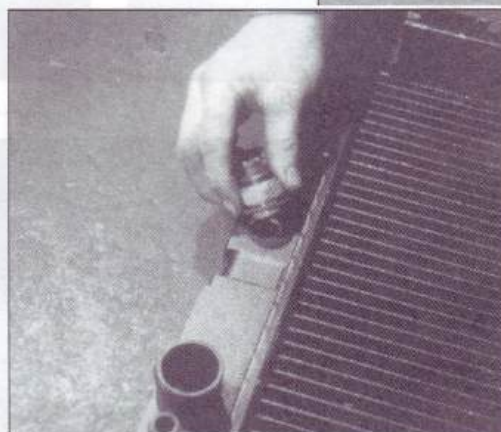
Fig.10b. Fitting the fan control switch.
