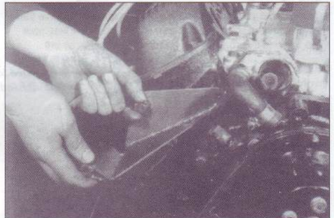
Fig.8n. Alternator mounting bracket being fitted to engine block. (Ford Small Block Windsor version illustrated)
