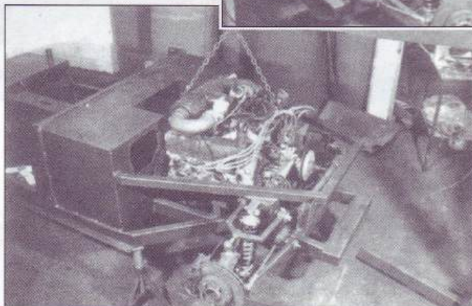
Fig.7d. Engine in position in chassis.
