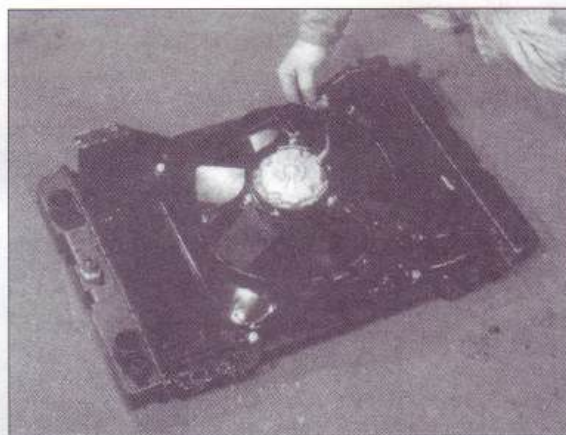
Fig.10d. Fan unit fitted to radiator
