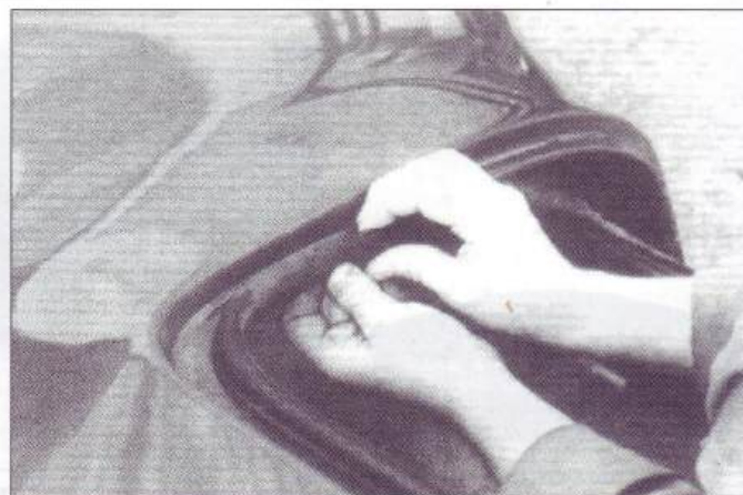
Fig.9l. Fitting the seal to the boot edge.
