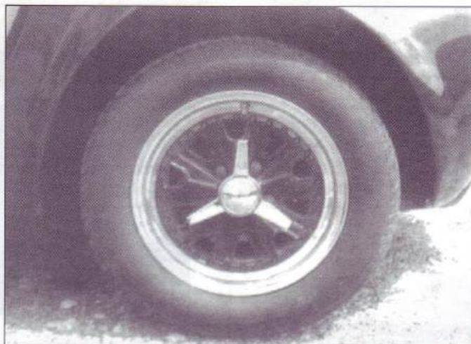
Fig.14a. Road wheel fitted. (Replica Halibrand type with dummy spinner illustrated)
