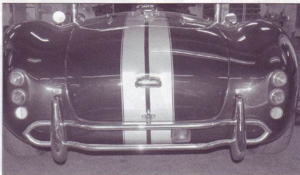
Fig.8j. Overriders and nudge bar assembly fitted.
