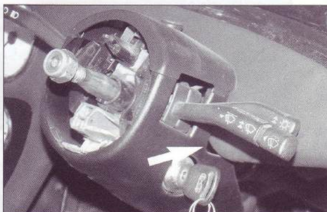
Fig.3a. Cowls trimmed and fitted
