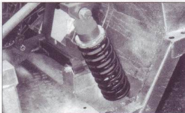
Fig.3g. Shock absorber fitted to chassis bracket.
