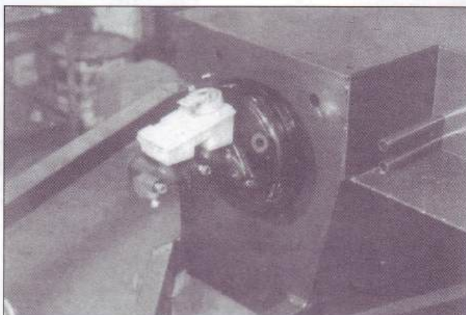
Fig.9b. Master cylinder / servo mounted to bulkhead.
