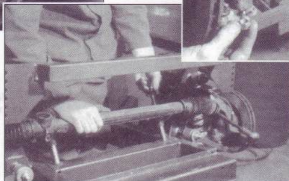
Fig.2q. Temporarily fitting rack and checking track rod taper fit (inset)
