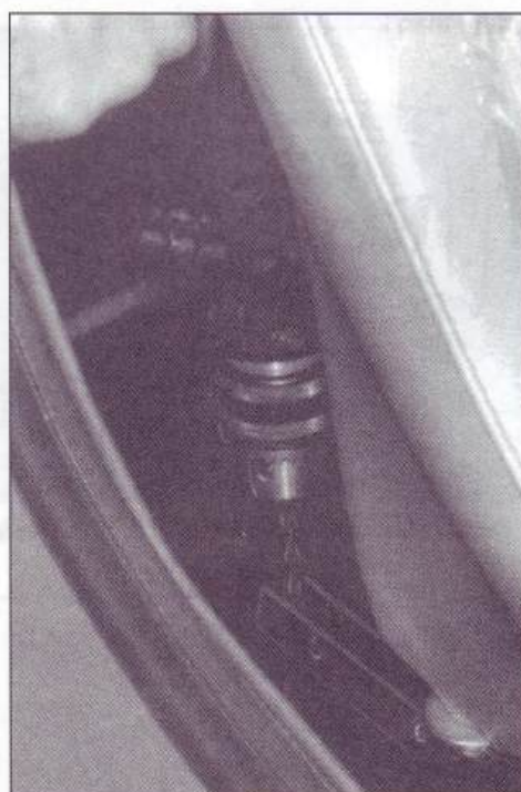
Fig.7c. Drilling seat fixing holes.
