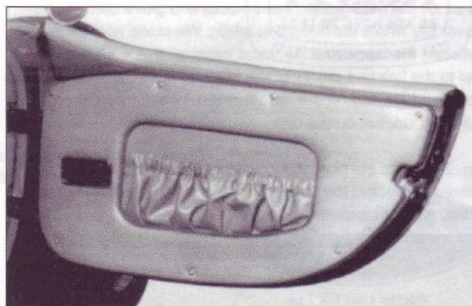
Fig.5a. Door trim panel fitted.
